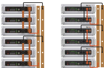
Figure 5-1 Schematic diagram of power cable connection
